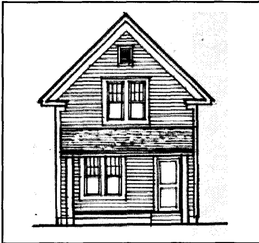
Appropriate: Window openings and trim are proportional to building and solid wall surface.
