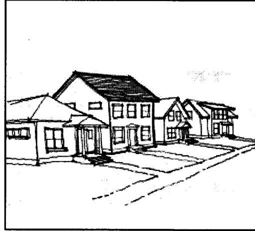
Inappropriate Infill: Roof forms are not compatible; large unbroken surfaces.
