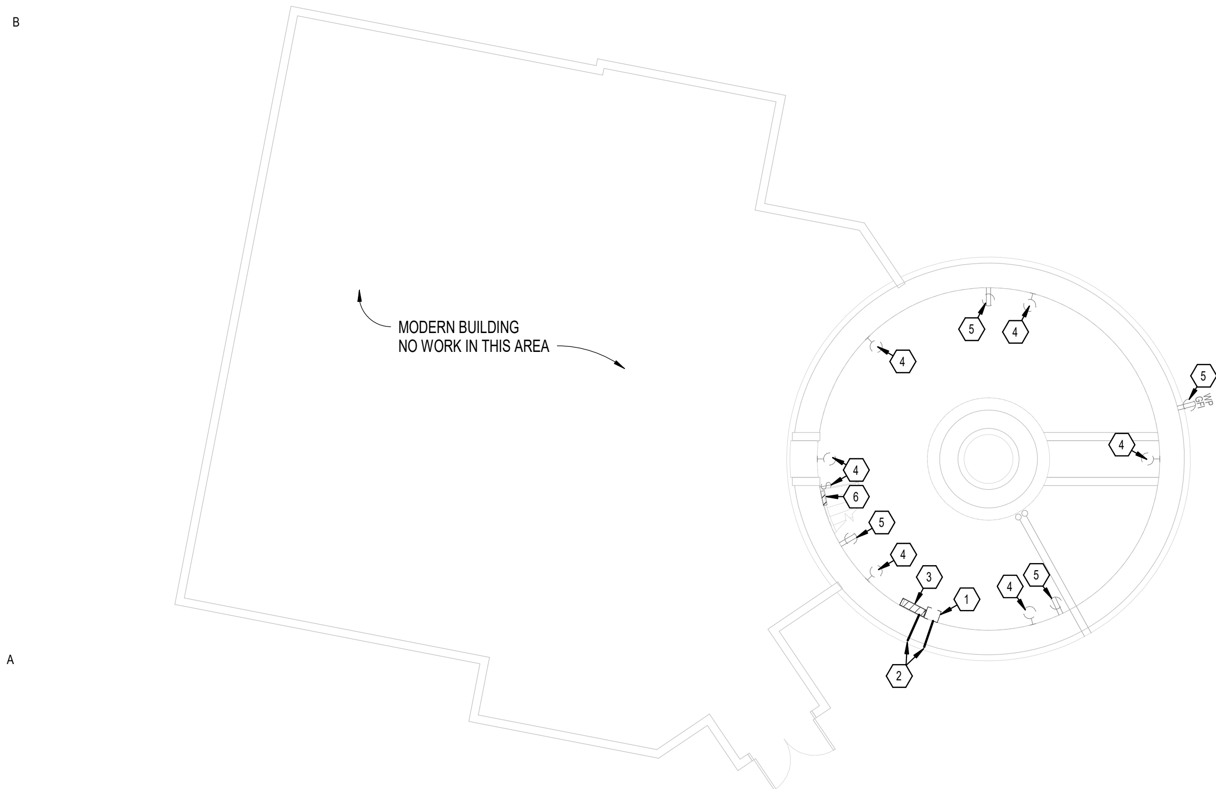
1 GROUND LEVEL - ELECTRICAL DEMOLITION PLAN
