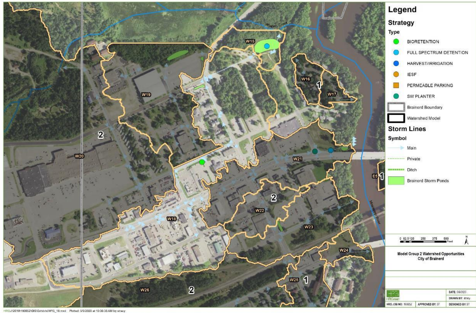
Figure 3. Subwatersheds W15 and W18 BMPs
