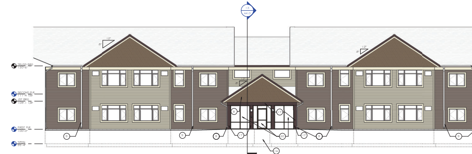
37 EXTERIOR ELEVATION - AREA D - NORTH 1/8" = 1'-0"
