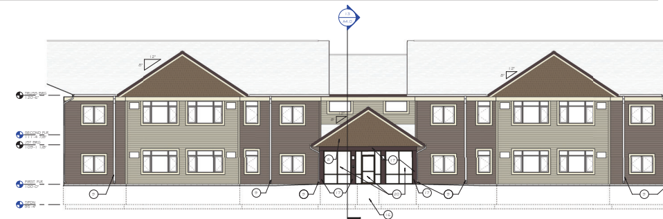
37 EXTERIOR ELEVATION - AREA D - NORTH 1/8" = 1'-0"
